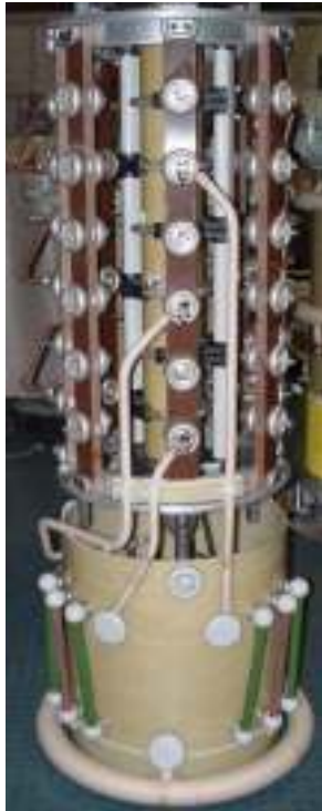
Tie-in resistor (and potential switch) mounted on a cylinder under the tap selector (OLTC type M/RM/VRC/VRE),
