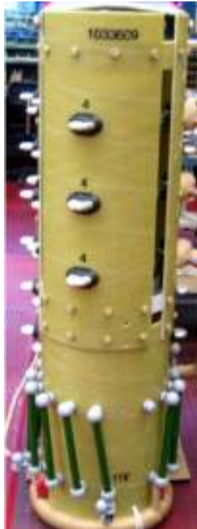
Tie-in resistor (and potential switch) mounted on a cylinder under the pre-selector (OLTC type R/VRD/VRF),
